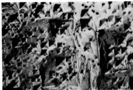
Fig. 3. Point-bottomed pyramidal pits developed in vacuum after 30 minutes at 680^{\circ}\text{C} ( \times 225 ).
