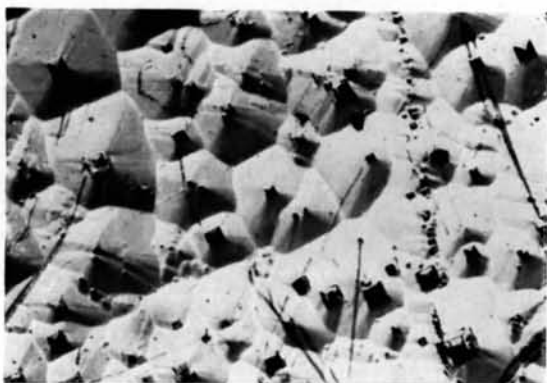
Fig. 4. Example of a strongly thermally etched crystal. 1 hour in vacuum at 725°C ( \times 225 ).
