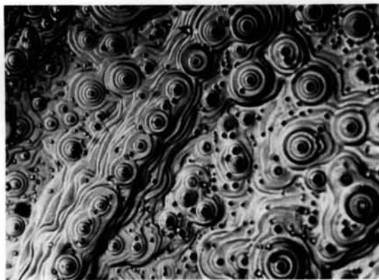
Fig. 2. Circular pits developed at 700^{\circ}\text{C} in air. Etching time of 1\frac{1}{2} hours ( \times 225 ).
